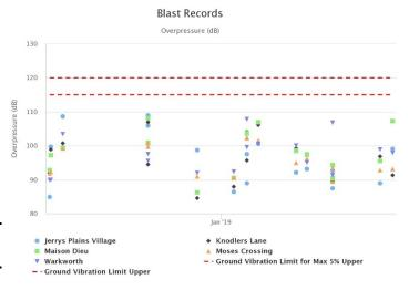
Figure 10: Overpressure Blast Monitoring Results – January 2019
